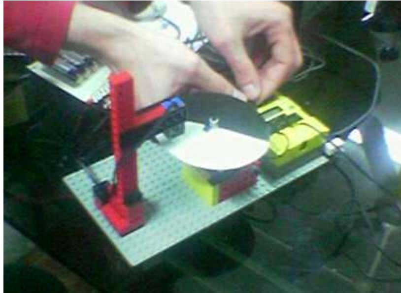
Figure 6. Students' construction to measure the rotation speed of the motor
